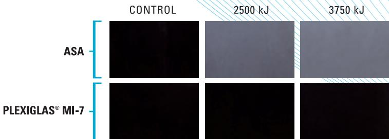
*After 3750 kJ exposure, the Plexiglas® sample still provides a deeper, jet-black appearance than is initially attainable with the competitive materials.*
